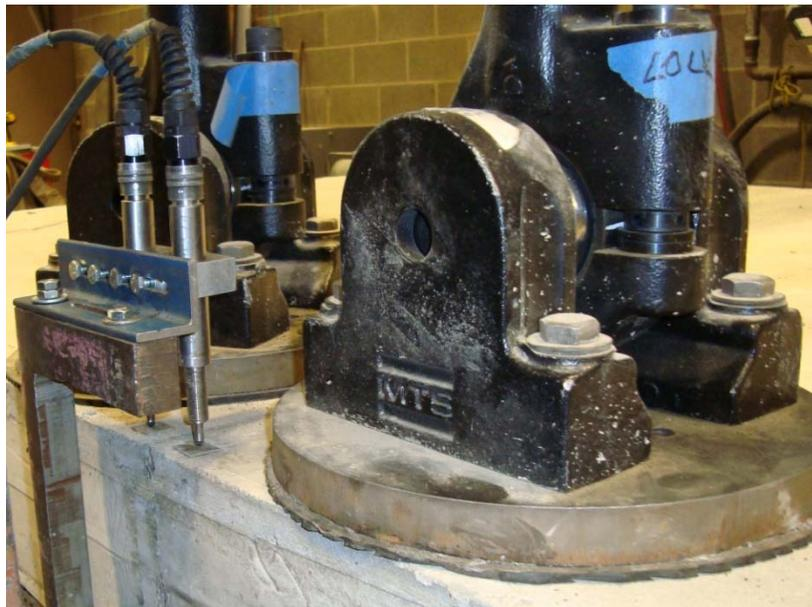
Figure 3. Photo of load plate and LVDT placement for the University of Pittsburgh dowel/slab test program (Vandenbossche, 2017).
