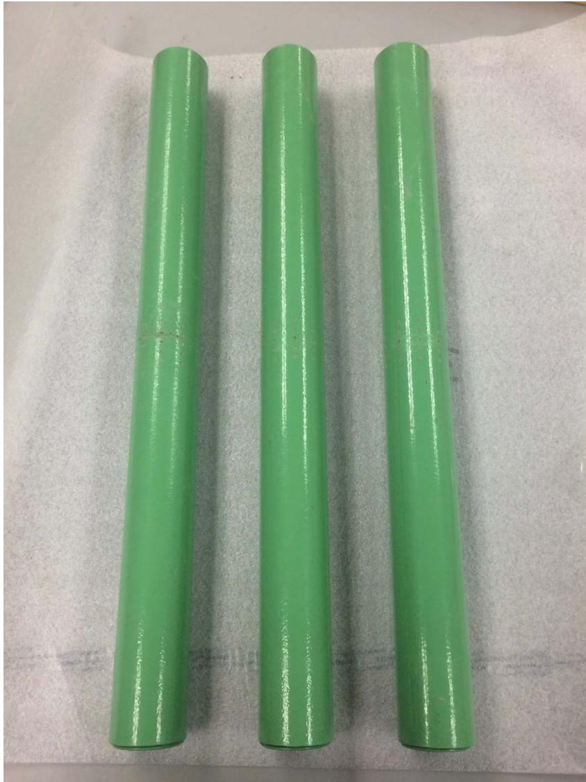
Figure 14. Photo of O-Dowels after completion of test and extraction from test panel.
